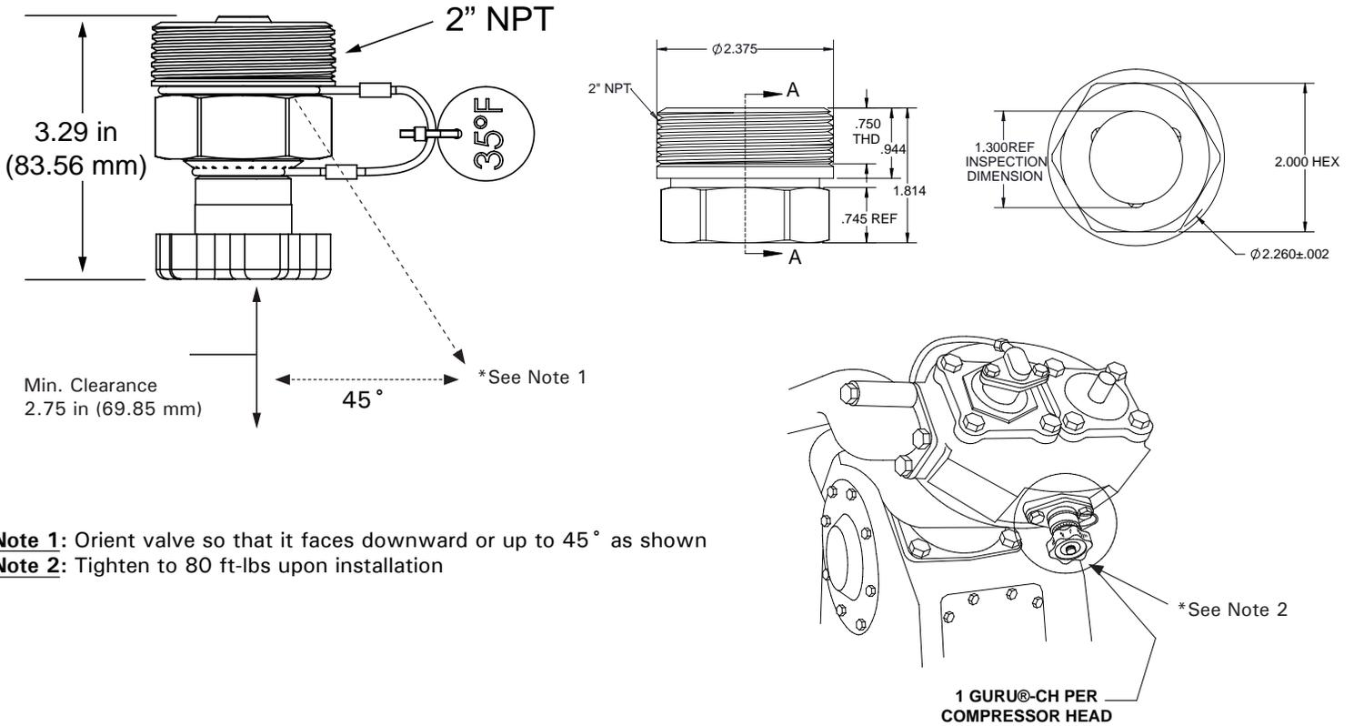
**Note 1:** Orient valve so that it faces downward or up to 45° as shown
